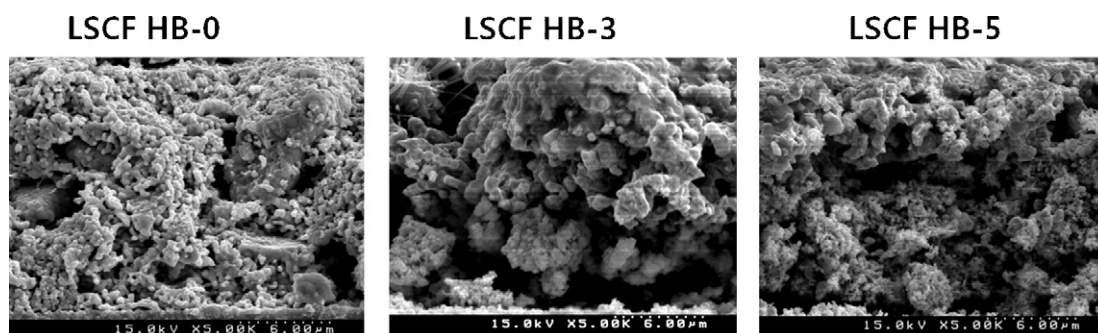
Fig. 5. Microstructures of cathodes with synthesized LSCF powders.
